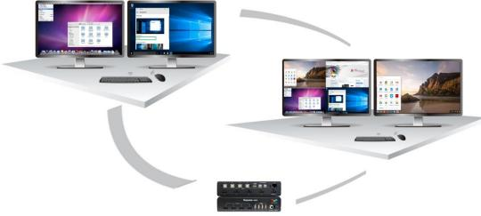
With two operators, each two-monitor workstation can be controlled with one keyboard and mouse, and an output can connect to a shared monitor, as shown in the example above.
